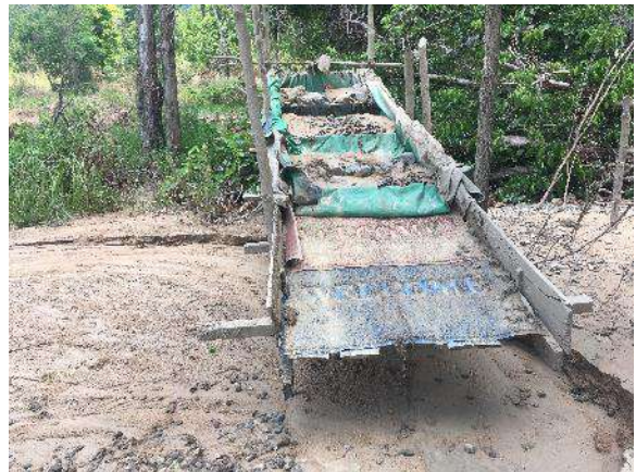
Gold Mining #15. Active alluvial artisanal gold mining (hydraulic mining). Sluce box.
