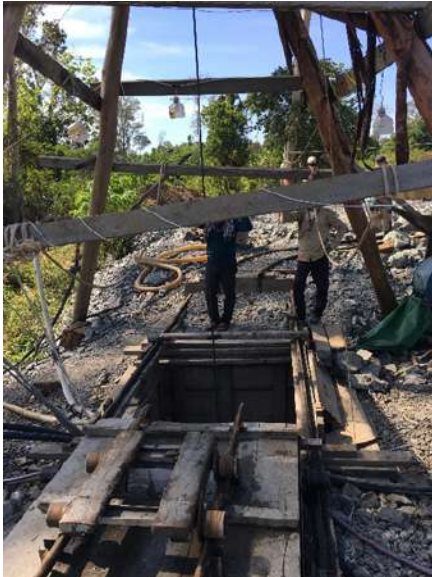
Figure 5. Gold hard-rock shaft mine to the northeast of Snang An Village (“Chinese mine”). Planet satellite image of mine area, late January 2019 (above). On-the-ground photo of mine shaft headframe, December 2018 site visit (upper left).
