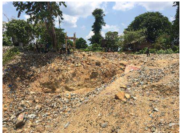
Gold Mining #3. Tailings above mine entrance.
