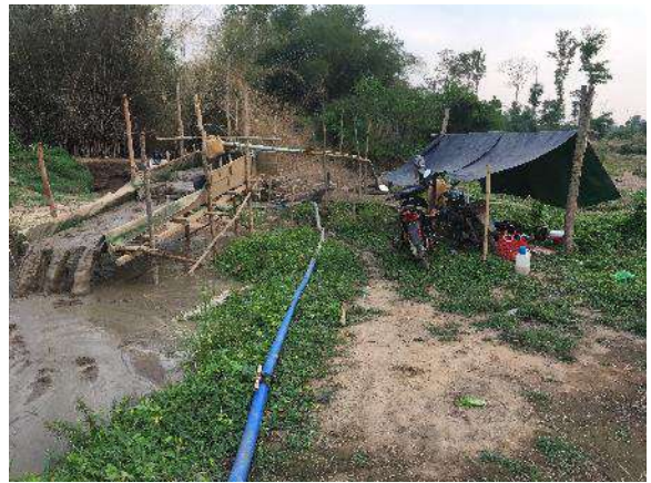
Gold Mining #10. Active alluvial artisanal gold mining (sluice box).
