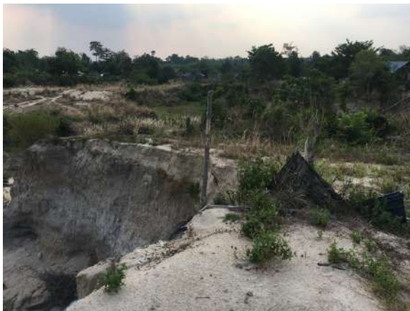
Gold Mining #8. Active alluvial artisanal gold mining in stream (hydraulic mining) just north of Phnom Chi.
