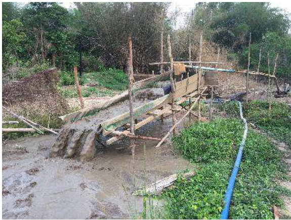
Gold Mining #10. Active alluvial artisanal gold mining (sluice box associated with hydraulic mining in above images).
