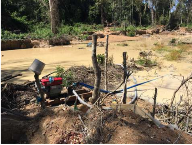
Photos on this page show Gold Mining Location #3, 2018, including hydraulic mining equipment (hoses, engines) and sluice boxes used for gravity separation of gold.
