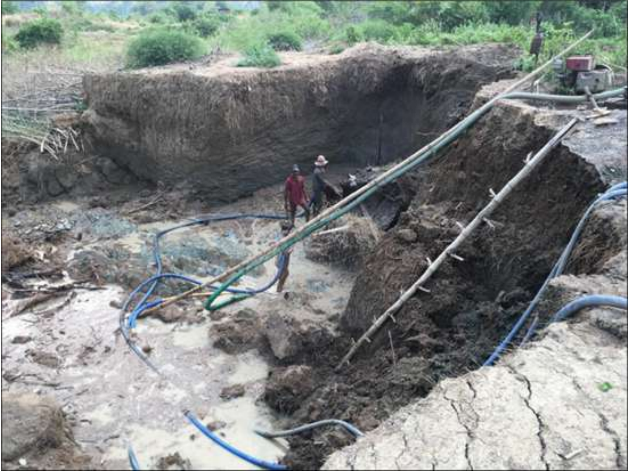
Figure 4. Photo illustrating artisanal gold mining of alluvial stream deposits using hydraulic (high-pressure jet of water) methods. This stream is located just northwest of Phnom Chi Mountain (shown in Figure 16).
