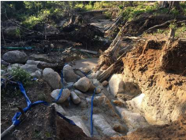
Hydraulic alluvial mining in streambed.
