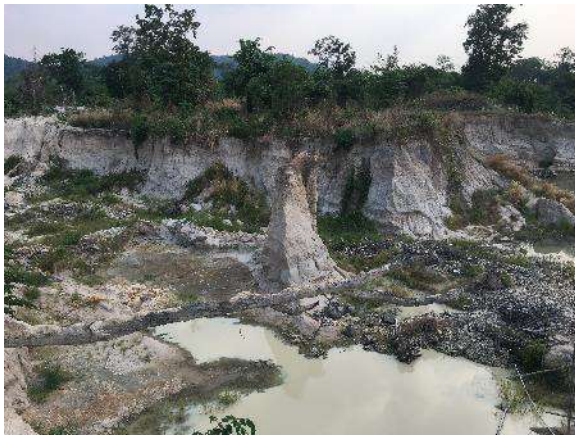
Gold Mining #8. Active alluvial artisanal gold mining showing impact of hydraulic mining on stream.
