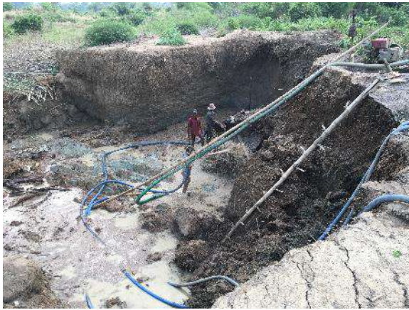
Gold Mining #10. Active alluvial artisanal gold mining (hydraulic mining active in pit).
