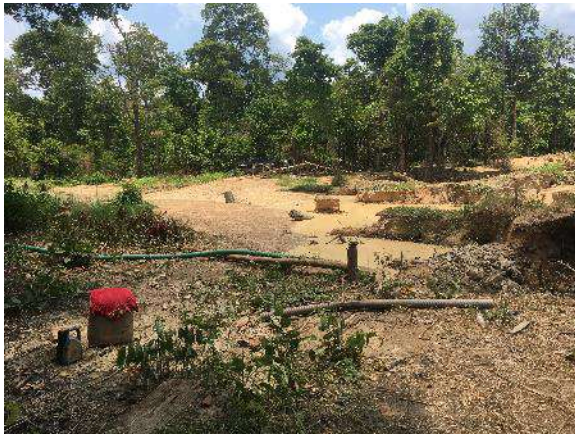
Gold Mining #15. Active alluvial artisanal gold mining (hydraulic mining). Sluce box visible in distance.
